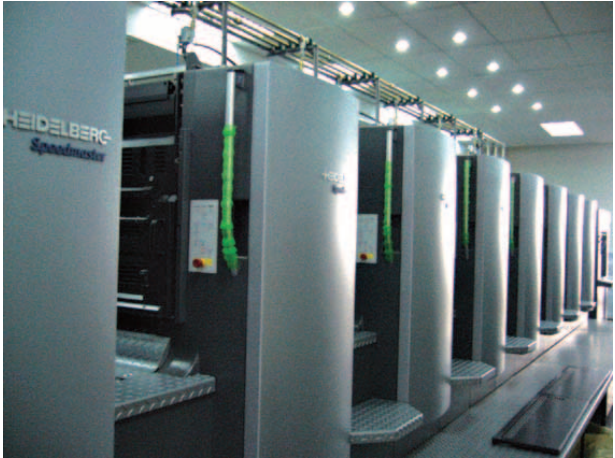
Heidelberg SM-102-8P (8-colour perfecter sheet-fed printing machine)
