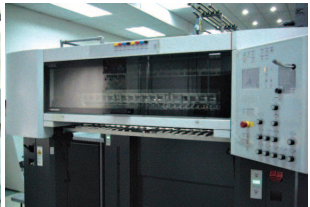
Heidelberg SM-102-8P (8-colour perfecter sheet-fed printing machine)
