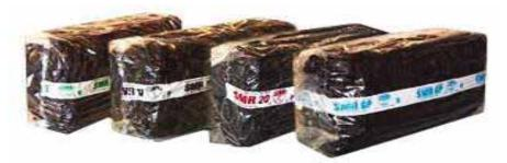
The different grades of SMR are produced by controlling the quality of raw materials input (e.g. dry rubber content of cup lump) and the drying process. Further details on the processing of block rubber are as set out in Section 7.4.1 of this Prospectus. The grading of SMR is based on the following parameters:
