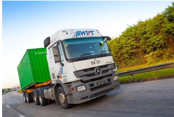
One of our prime movers hauling a 40-foot container on a container trailer
