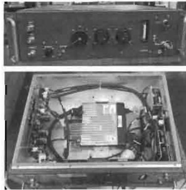
System build finished product - train communication interface unit
