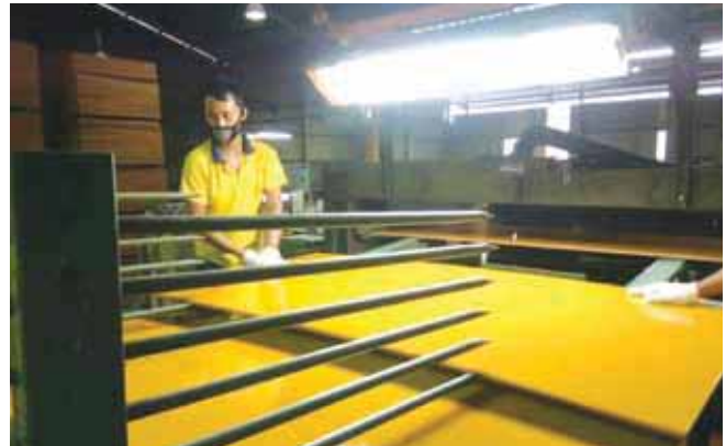
Coated Concrete Panel (CCP) Grading
