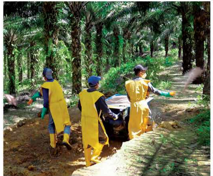
Power barrow for ease of FFB evacuation in terraced areas and also for fertiliser application.
