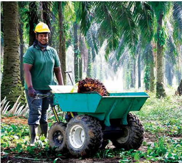
Power barrow for ease of FFB evacuation in terraced areas and also for fertiliser application.
