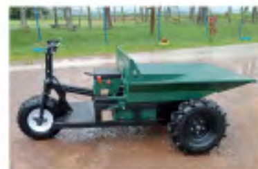
Electric Mechanical Cart: Assist in transporting and evacuation of FFB in the plantations
