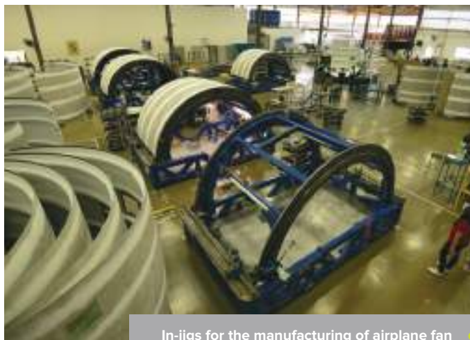
In-jigs for the manufacturing of airplane fan cowl doors in the CTRM plant
