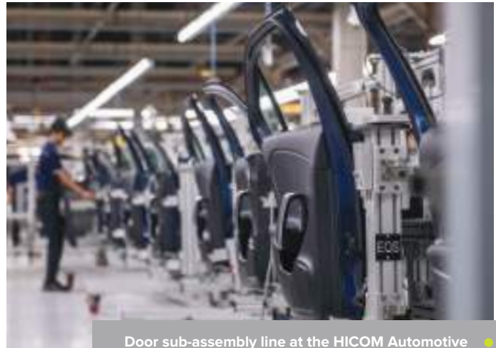
Door sub-assembly line at the HICOM Automotive Manufacturers (Malaysia) plant in Pekan, Pahang
