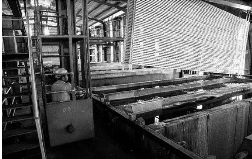
Preparing to submerge the extruded aluminium profiles into the anodising solution
