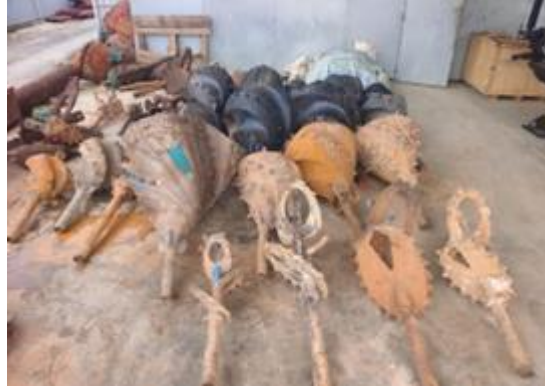
Reamer units of varying sizes affixed to HDD machines to enlarge pilot bore
