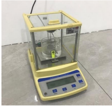
Electronic densimeter used for density test (maximum 200 grams)
