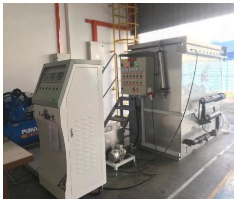
Hydrostatic pressure testing machine used for hydrostatic test (0 – 20 megapascal)
