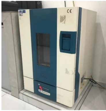
Forced convection oven used for longitudinal reversion test (maximum 250°C)
