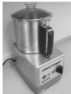
Robot coupe cutter mixer used for cutting and blending food ingredients to form consistent food ingredients mixture
