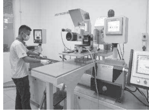
Our lab-scale twin screw extruder with pelletiser used for product development of bioplastic compounds
