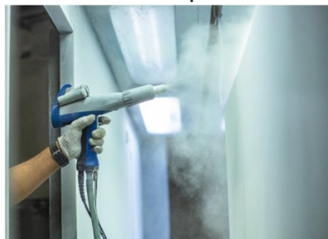
Powder coating process for our fabricated parts
