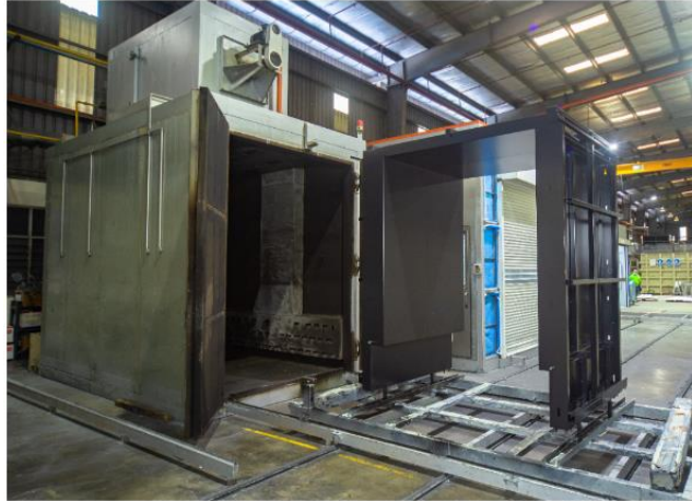
Our powder coating line incorporating powder spraying and oven
