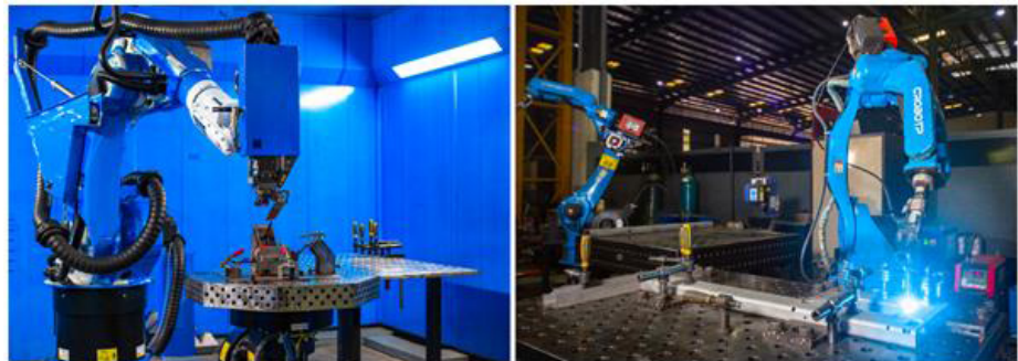
Left: CNC robotic-arm laser welding machine; Right: CNC robotic-arm MIG welding machine
