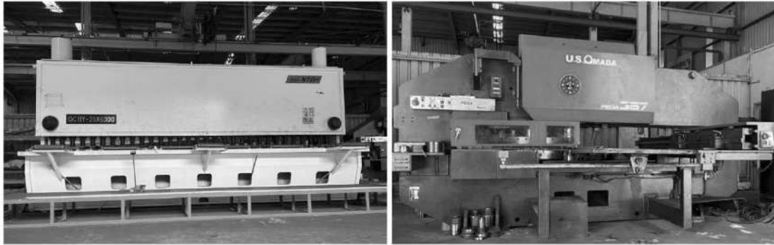
Left: A cutting machine; Right: A punching machine
