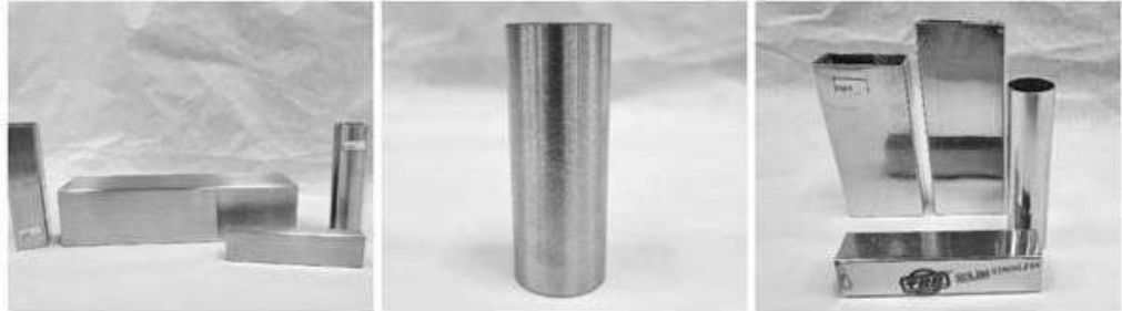
Left: 180 grit (ground finish); Middle: 320 grit (dull finish); Right: 600 grit (bright polish)
