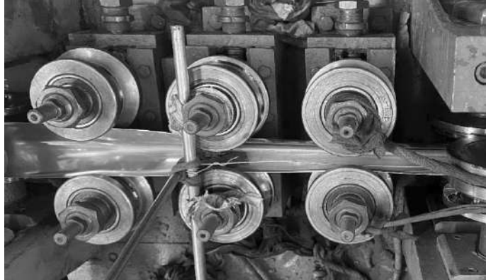
Forming process for a tubular section
