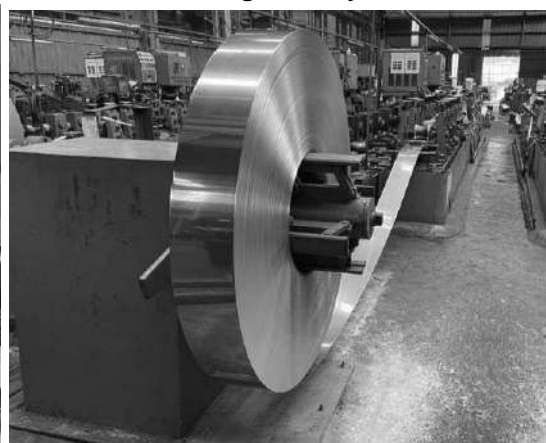
Decoiling the baby coil
