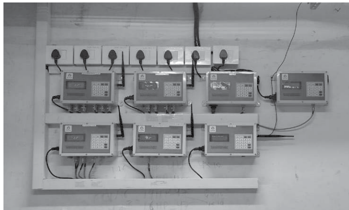
Wireless sensor modules
