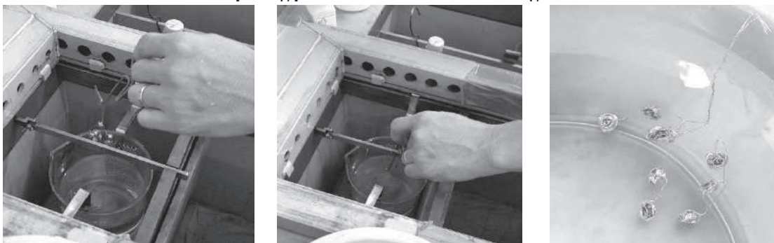
Electroplating process to make rose coloured gold item
