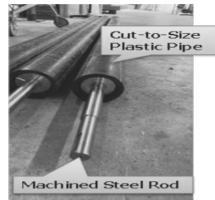
Cut-to-size plastic pipe inserted to machined steel rod
