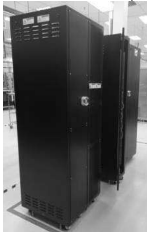
Telecommunications frame, structure and enclosure, after sub-module assembly
