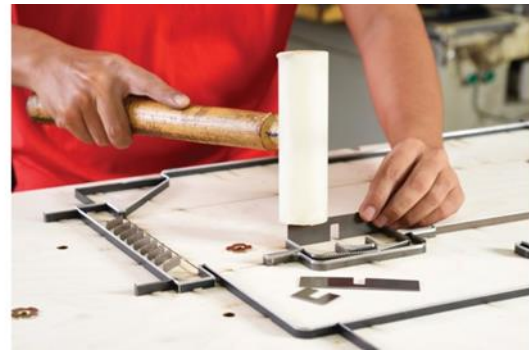
Steel rules mounting (Flatbed die-cutting mould)
