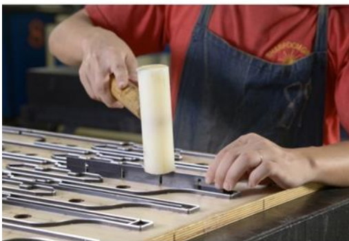
Steel rules mounting (Flatbed die-cutting mould)
