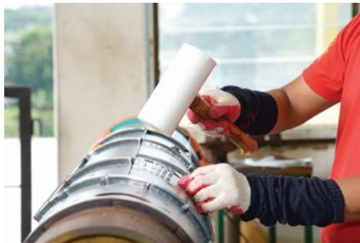
Steel rules mounting (Rotary die-cutting mould)
