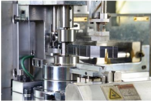
Automatic steel rule processor
